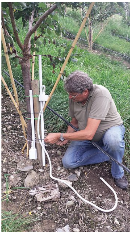
Fig. 4. Philippe Monney from the Agroscope Research Station in Conthey/VS setting up the EnvEve SA monitoring system in an experimental apricot orchard.
